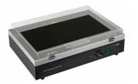
High Performance 2UV models are the same size and design as other high performance models but are equipped with midrange (302 nm) and longwave (365 nm) UV in each unit.  Deliver high UV output and intensity, no light flicker, fast lamp start-up and reduced electrical consumption
